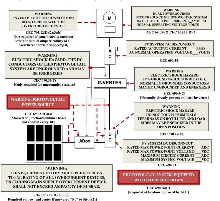
Informational note: ANSI Z535.4 provides guidelines for the design of safety signs and labels for application to products. A phenolic plaque with contrasting colors between the text and background would meet the intent of the code for permanency. No type size is specified, but 20 point (3/8") should be considered the minimum.
