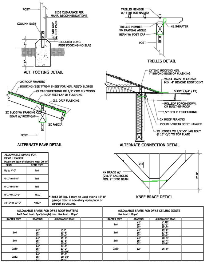
TYPE V CONSTRUCTION IS A CLASSIFICATION OF BUILDINGS BY CONSTRUCTION MATERIALS AND METHODS. IT IS THE LEAST RESTRICTIVE PERMITTED BY THE UNIFORM BUILDING CODE AND INCLUDES LIGHT, WOOD-FRAME CONSTRUCTION. THIS SHEET IS FOR INFORMATION AND REFERENCE ONLY AND IS NOT A SUBSTITUTE FOR ACCURATE DRAWINGS PREPARED FOR EACH PROPOSED CONSTRUCTION PROJECT.
