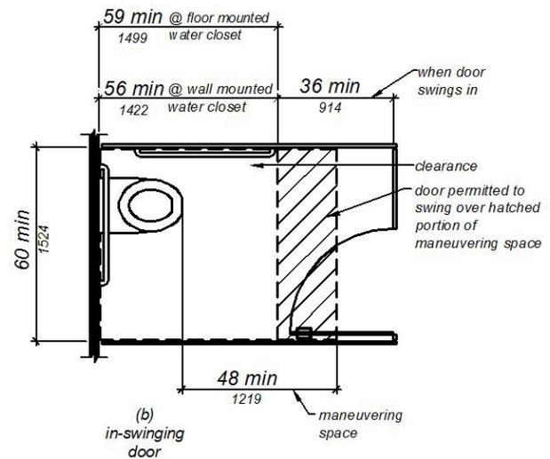
**FIGURE 11B-604.8.1.1.3 - MANEUVERING SPACE WITH END-OPENING DOOR**
