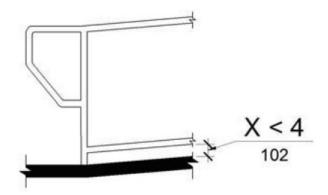
FIGURE 11B-405.9.2 CURB OR BARRIER EDGE PROTECTION
