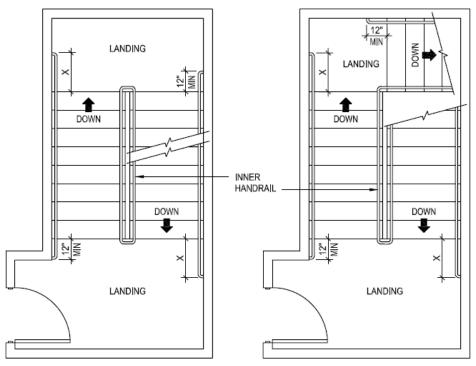
NOTE; INNER HANDRAIL AT LANDINGS OF STAIRS THAT DOUBLE BACK OR IMMEDIATELY TURN SHALL BE CONTINUOUS AND SHALL NOT EXTEND INTO LANDING OR ACCESSIBLE ROUTE OF TRAVEL
