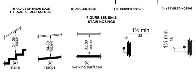
FIGURE 11B-505.4 HANDRAIL HEIGHT
