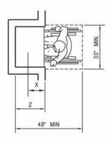
NOTE: X SHALL BE LESS THAN OR EQUAL TO 25 INCHES Z SHALL BE GREATER THAN OR EQUAL TO X. WHEN X IS LESS THAN 20 INCHES, THEN Y SHALL BE 48 INCHES MAXIMUM. WHEN X IS 20 TO 25 INCHES, THEN Y SHALL BE 44 INCHES MAXIMUM.
