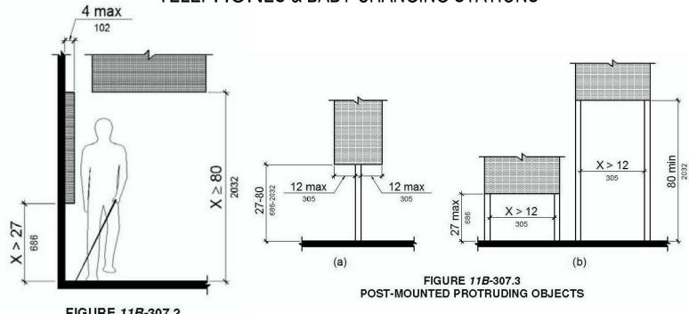
FIGURE 11B-307.2 LIMITS OF PROTRUDING OBJECTS
