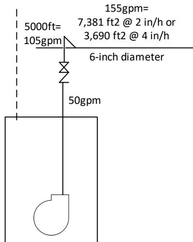
at 2 in/h rainfall, 50 gpm are equivalent to  $50/0.021=2381 \text{ ft}^2$  (Table D101.1)
